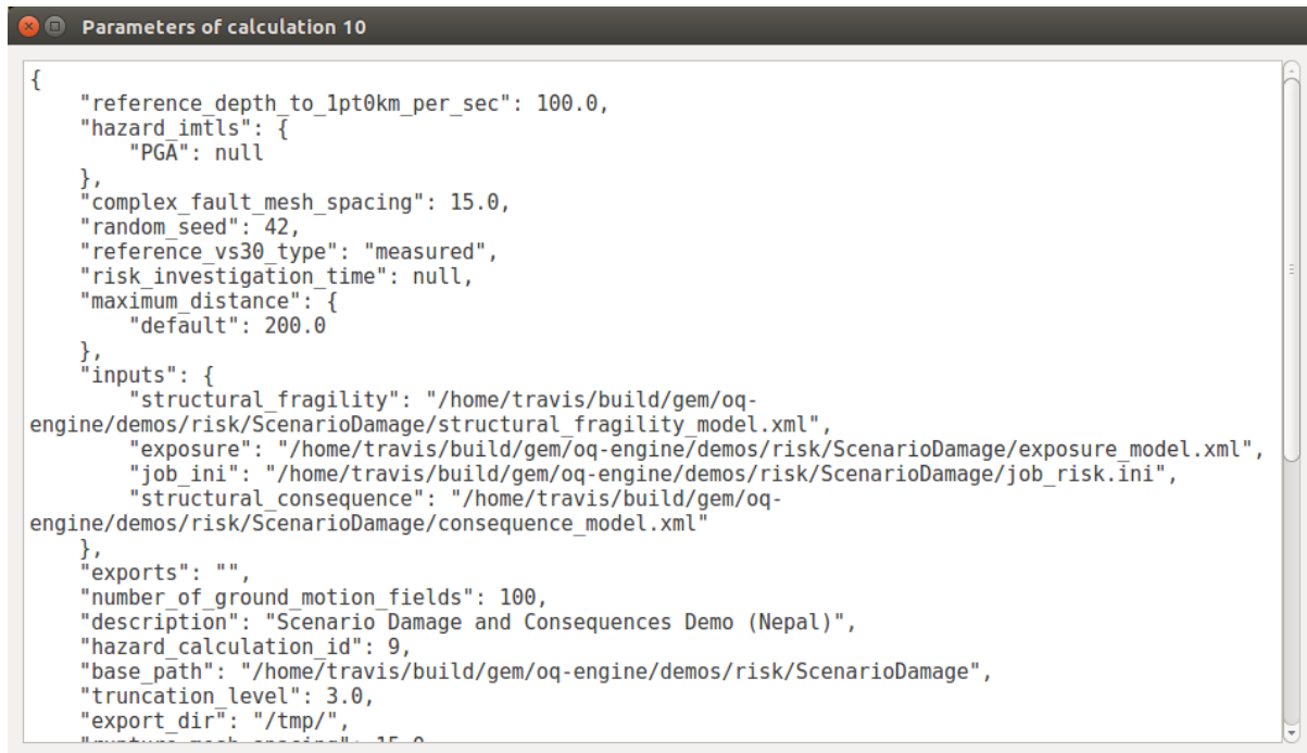
Fig. 15.3: Example showing parameters of a OQ-Engine calculation
