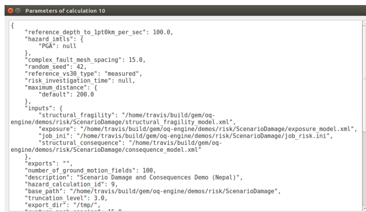
Fig. 15.3: Example showing parameters of a OQ-Engine calculation
